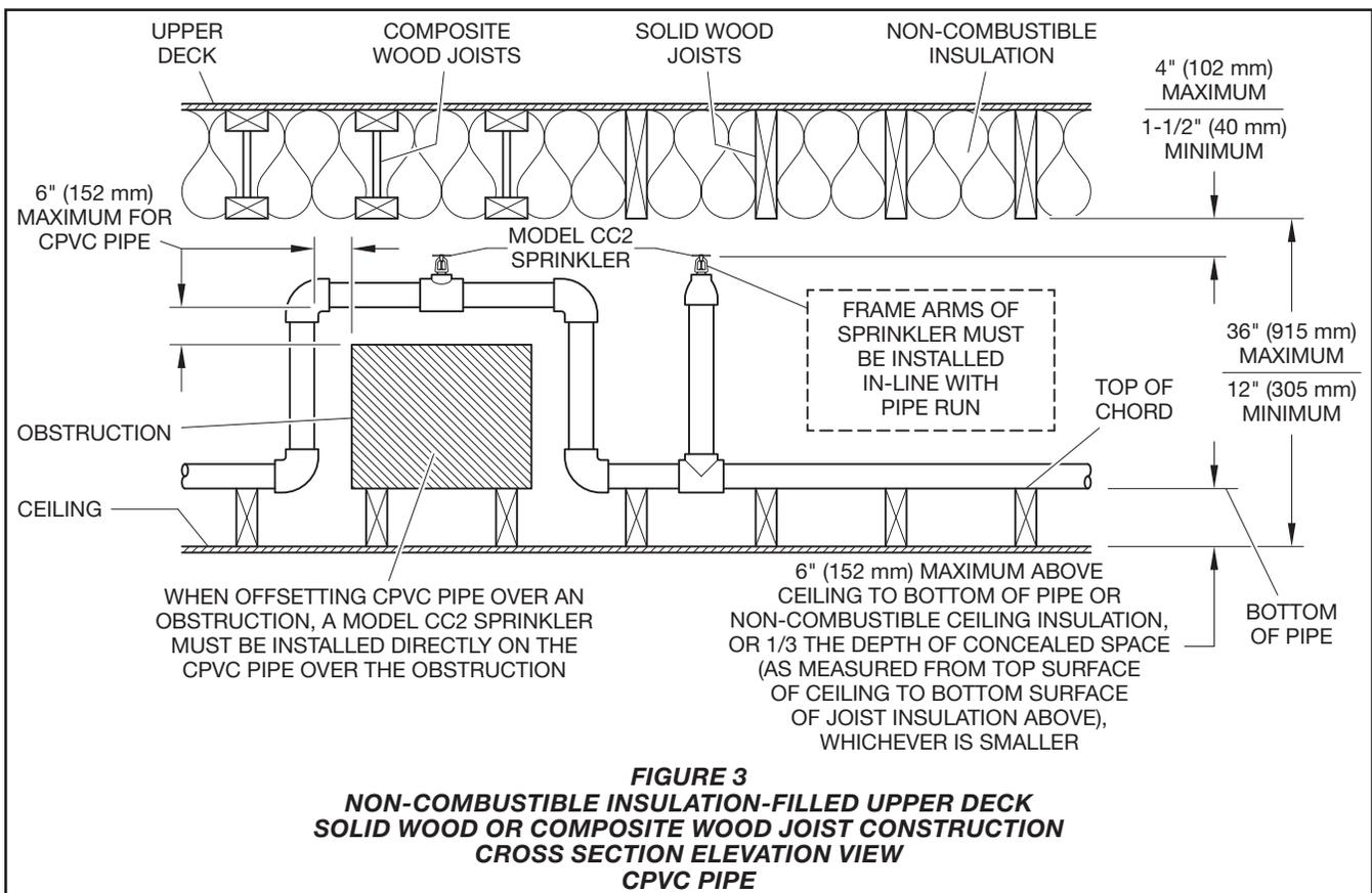
1 in. (DN25) or larger pipe, a hanger must be located at the truss nearest a sprig for purposes of restraint. If using 3/4 in. (DN19) piping, all sprigs over 12 in. (305 mm) must be laterally braced using methods described in the NFPA standards.
